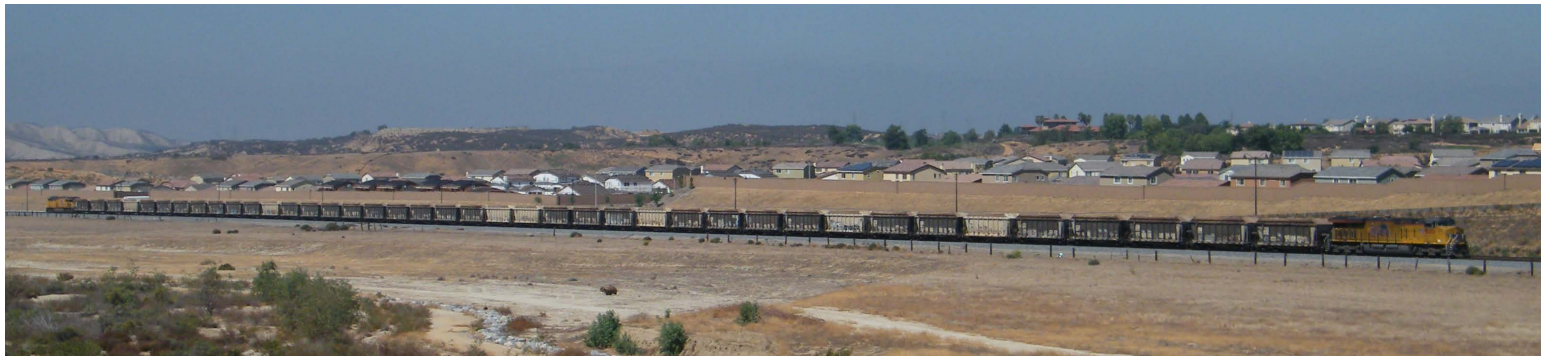
The rock train that had just left the quarry in Cabazon. This was pretty neat to see. This train is ran with power on each end signifying that it is ran point to point with no area to turn engines around. I was particularly happy to see it as it reminded me of the coal trains that run up into Yankeetown with NS power on them; one locomotive at each end.
